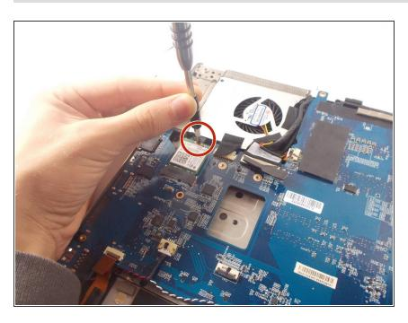
Use the screwdriver to unscrew the 0.5mm Phillips #0 screw holding the Wi-Fi card in place.
