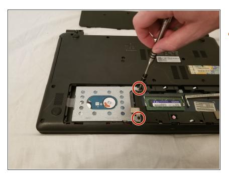
Unscrew the two CM2\*3-4 screws that attach the hard drive to the Laptop.
