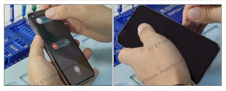
Press the wake button and volume down button to turn off the phone.
