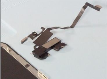
Undo 3 Y000 screws and heating the flex cable with a heat gun, we can remove the ear speaker easily
