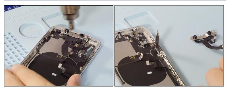
• Heating the front facing camera with a heat gun will make it easily to be removed
