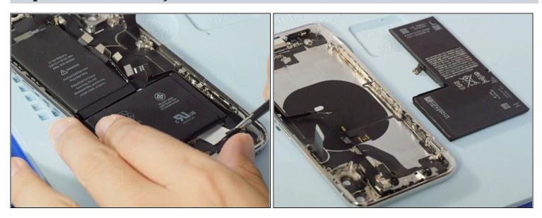
• Pulling out 4 battery adhesives with a <u>tweezers</u> then we can remove the battery.
