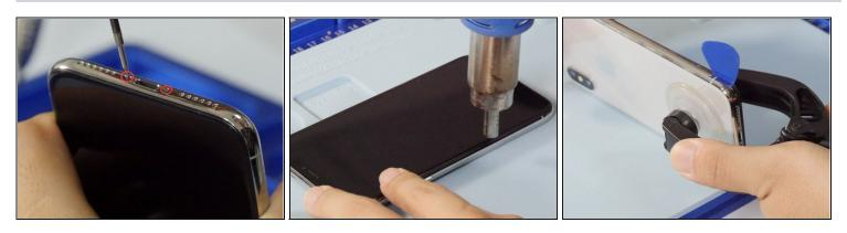
• Use the Pentaloble screwdriver to remove the charging port screws. Heating the phone with a heat gun will allow the phone to be opened more easily.
