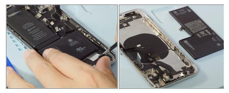
• Pulling out 4 battery adhesives with a tweezers then we can remove the battery.
