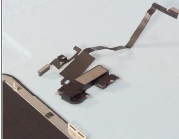
Undo 3 Y000 screws and heating the flex cable with a heat gun, we can remove the ear speaker easily
