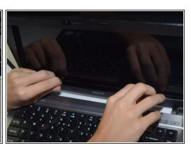
Carefully pull the bevel (frame) off of the screen
