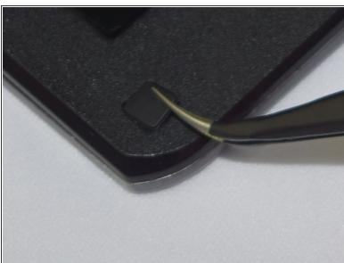
Locate and remove the four (4) pads using Angled Tweezers
