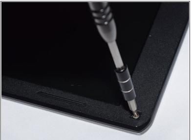
Remove the four screws that were under the pads
