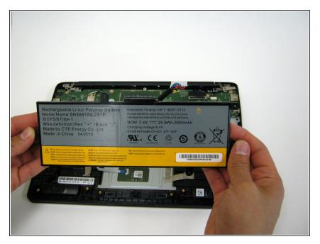
Lift the battery from the frame.
