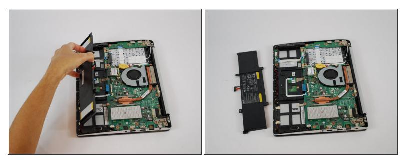
• Gently remove the battery from the slot.
