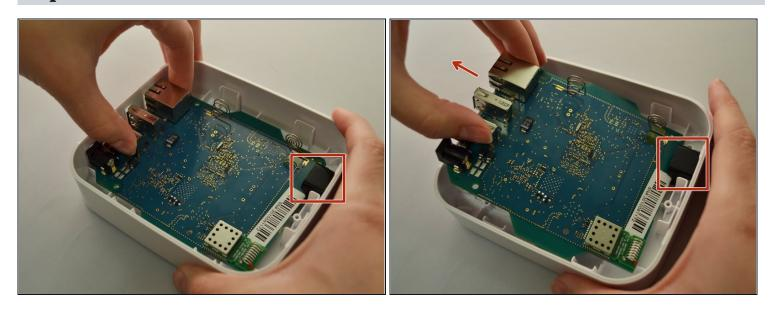
• To remove the motherboard, grip the USB port and the Ethernet port. Lift up, then slide towards the front of the device to release the motherboard from the black retaining clip shown on the right.
