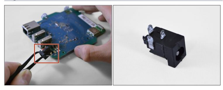
• Using <u>tweezers</u>, remove the desoldered power port from the motherboard.
