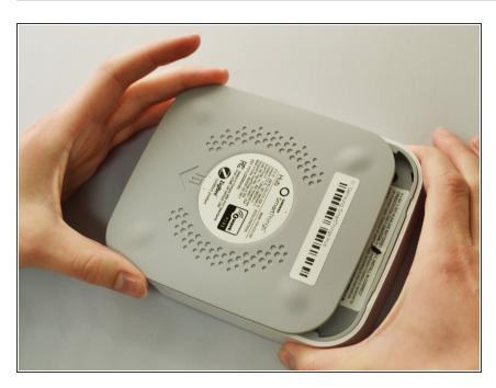
To open your device, gently slide the grey bottom cover in the direction of the arrow as shown.
