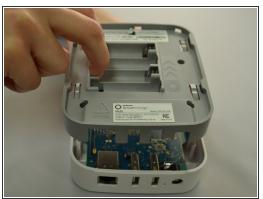
Once all five screws are removed, split the casing apart by applying gentle upwards pressure against the positive terminals in the battery compartment.
