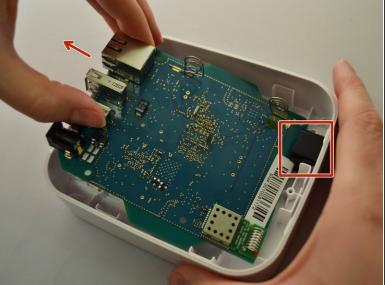
• To remove the motherboard, grip the USB port and the Ethernet port. Lift up, then slide towards the front of the device to release the motherboard from the black retaining clip shown on the right.
