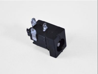
• Using tweezers, remove the desoldered power port from the motherboard.
