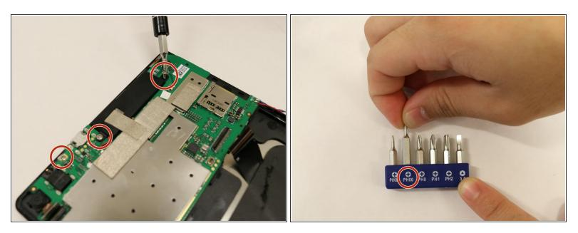
Remove the three 2.0mm screws using the Phillips #00 Screwdriver bit.
