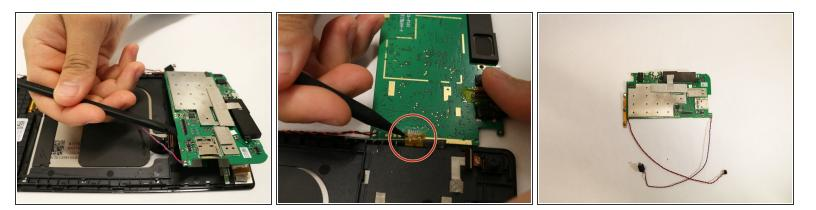
After taking out the twisted pairs, there is still one more strip that needs to be removed. It is located off the side of the motherboard and is the piece that receives input for volume and power.
