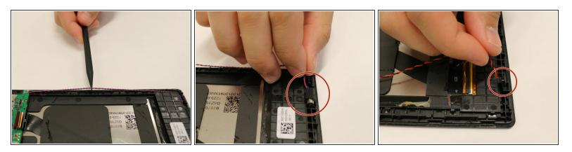
(i) There are two twisted pairs of wires on the left and right edges of the case.
