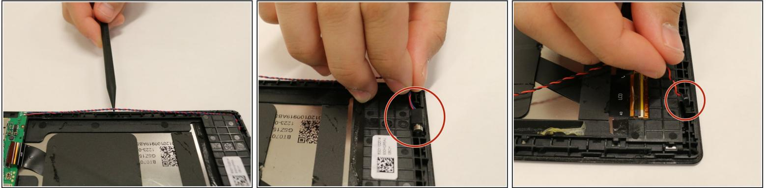
**i** There are two twisted pairs of wires on the left and right edges of the case.
