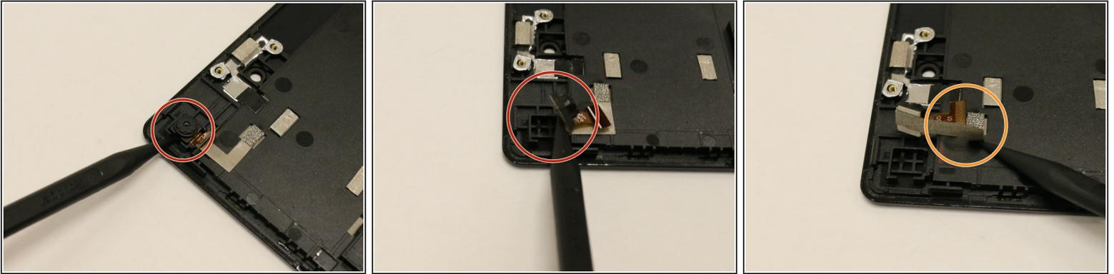
**i** The camera lens is located at top left corner of the back panel.
