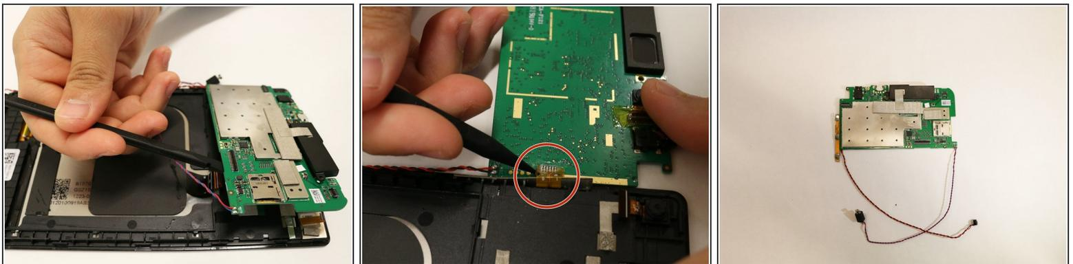
**!** After taking out the twisted pairs, there is still one more strip that needs to be removed. It is located off the side of the motherboard and is the piece that receives input for volume and power.
