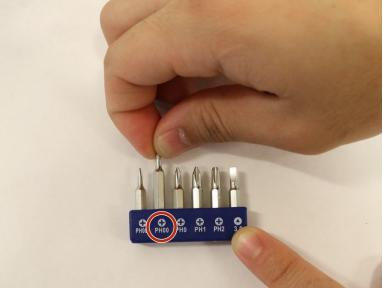
• Remove the three 2.0mm screws using the Phillips #00 Screwdriver bit.
