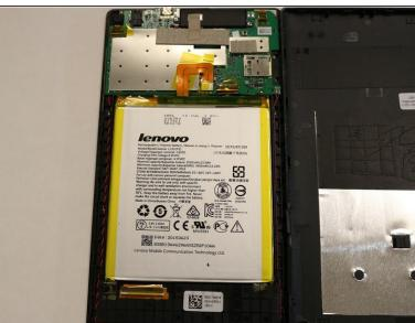
Starting at any point along the seam of the case carefully pry it open with the metal spudger, slowly
