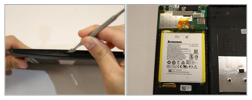
Starting at any point along the seam of the case carefully pry it open with the metal spudger, slowly
