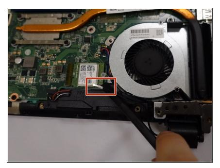
• Pull the cable from the clips and use the spudger to disconnect the wire from the Wi-Fi card.
