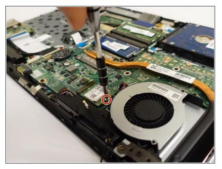
• Use the Phillips #1 screwdriver to remove the single 4mm screw.
