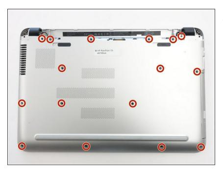
Remove the sixteen 8mm screws that hold the bottom cover with a Phillips #1 screwdriver.
