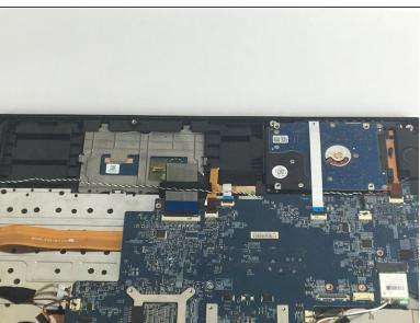
Unplug the battery connection carefully from the motherboard, and remove the old battery.
