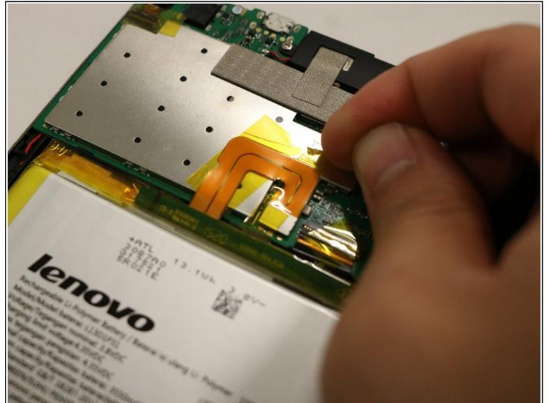
**i** The battery is connected to the motherboard by the thin wire shown here.
