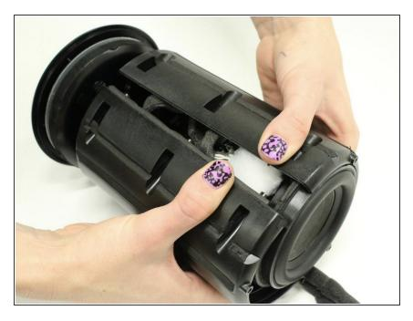
Open up the speaker body to expose the inner panel, and motherboard.
