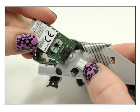
Press the white tab while gently pulling the Bluetooth module away from the connector and frame.
