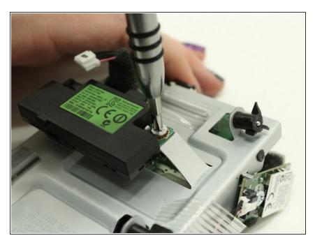
Remove the one PH2 Phillips screw from the WiFi module.
