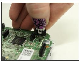
• Pinch the release tab on the remaining small white connector to disconnect the final wiring harness from the motherboard.
