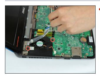
Unscrew the indicated 5.6mm screws with the #0 Phillips Head Screwdriver.
