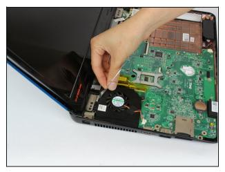
• Remove the fan from the device.
