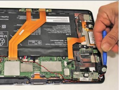
Use the narrow plastic opening tool to pry the speakers from the casing.
