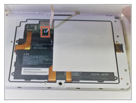
Carefully lift the back case and remove the smartcard ribbon from the motherboard.
