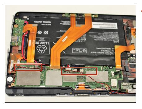
Pull up the cord that connects the battery to the motherboard
