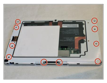
Remove the ten 3mm screws with a PH00 screwdriver from the shield.
