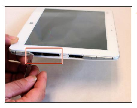
Close the slot cover by sliding the cover over the input slots and clipping into place.
