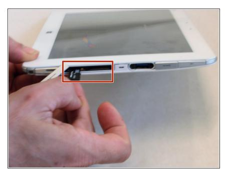
Pull the sim card out of the slot.
