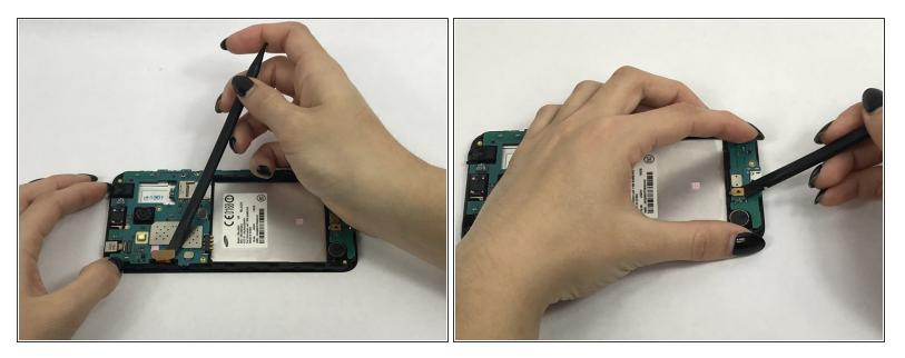
• Remove these connectors from the motherboard with spudger.
