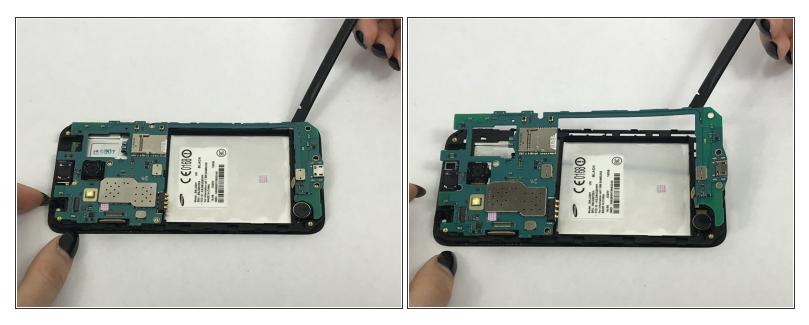
• Carefully use the spudger to pry the motherboard out of the plastic tabs.
