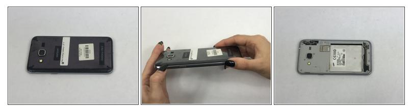
• Place your thumb on the top left corner and pry the tab open and lift off the back cover.
