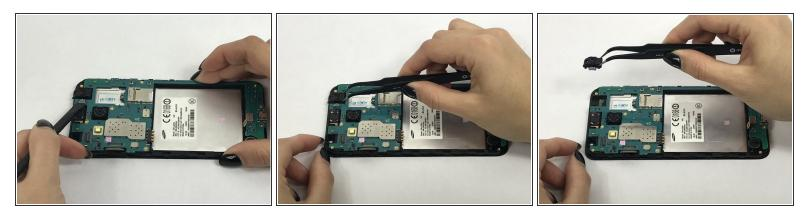
• Remove connector tab with spudger then carefully remove headphone jack with tweezers.
