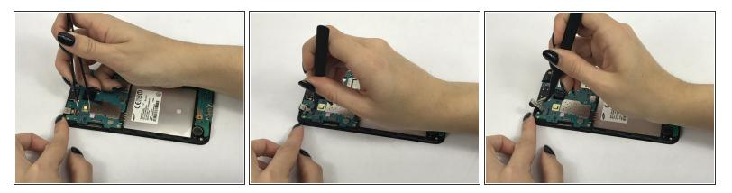
• Use tweezers to flip tab of the front camera to remove it.
