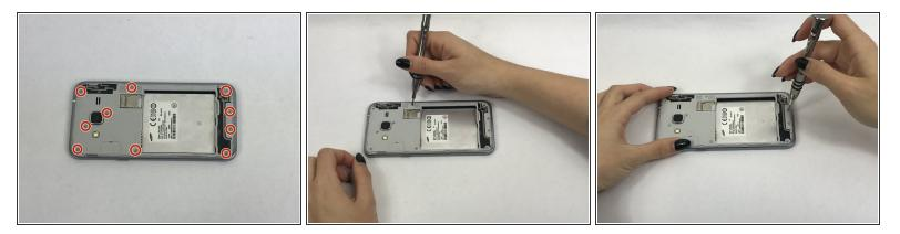
• Remove the ten 2.0 mm screws with the Phillips #J000 screwdriver.
