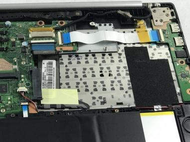
Remove the SSD (Solid State Drive) assembly from the upper case.
