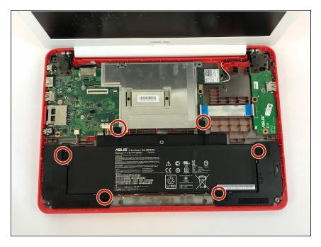
Using the JIS J0 Screwdriver, unscrew and remove the (6) six 6mm screws from the device.
