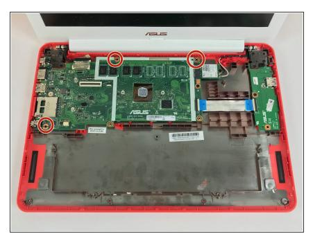
Using the JIS J0 Screwdriver, unscrew and remove the (3) three 6mm screws from the left hinge.
