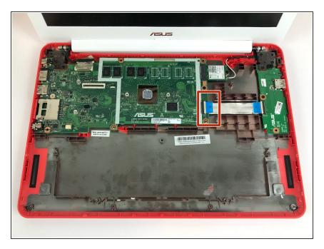
Using the plastic opening tool, lift up on data cable for the daughterboard to remove it from the device.
