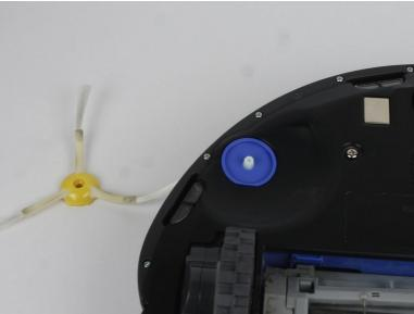
Flip the Roomba over and unscrew the side brush screw using the Phillips #2 screwdriver.
