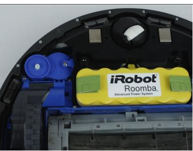
Unscrew the (4) four screws to the back plate and lift off.
