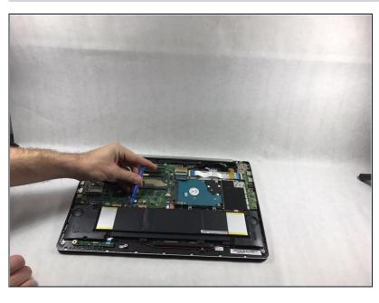
Use the flat end of the blue plastic opening tool to lift the battery connector up out of its socket on the motherboard.
