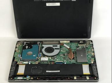
Slightly lift the lower case and push it toward the rear of the computer to free the mounting tabs.
