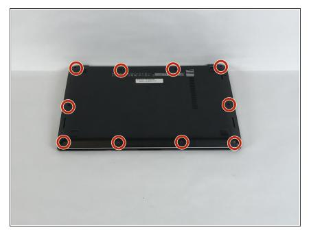
Unscrew the (10) screws on the bottom of the computer chassis using the JIS #0 screwdriver.
