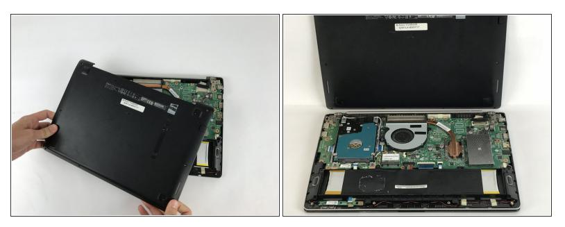
• Slightly lift the lower case and push it toward the rear of the computer to free the mounting tabs.
