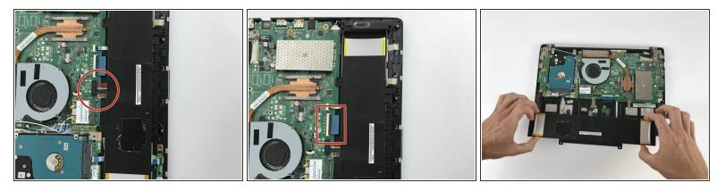
• Gently take the battery out of the laptop, making sure that all wires connecting to it are disconnected.
