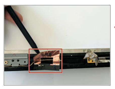
Remove the golden tape adhering to the display panel using a plastic spudger.
