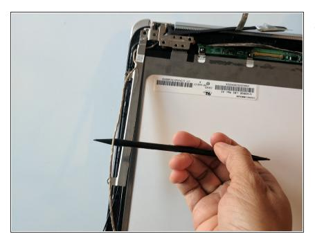
Remove the white color wifi antennas from the display panel using a plastic spudger.
