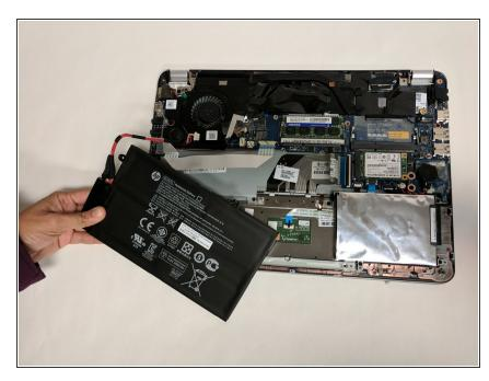
• Lift the battery up and remove.
