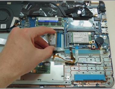
Remove the ribbon cable running from under the motherboard by undoing the latch mechanism with your fingernail, and pulling out on the edge of the connector. (This is the keyboard cable).
