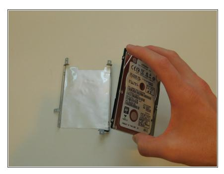
Remove the hard drive from the hard drive case.
