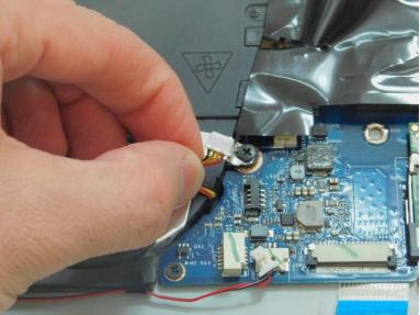
• Disconnect the multicolored power connector for the USB/audio board by first probing it gently with a plastic spudger, then pulling it free.
