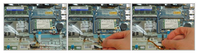
Disconnect the two small ribbon cables in front of the hard drive. The larger one is the touchpad board cable, and the smaller one is the keyboard light cable.
