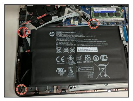
Unscrew and remove the three 4.0 mm Phillips-head screws that hold the battery in place, using a Phillips #1 screwdriver.
