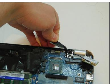
Using your fingers, locate the display panel cable under the hinge and disconnect it.
