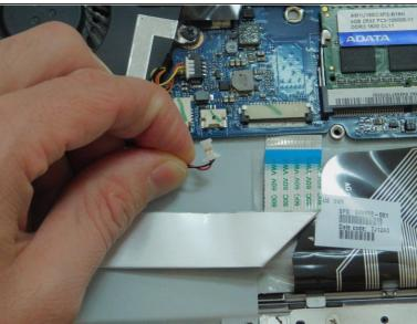
Disconnect the red and black power connector for the subwoofer by first probing it gently with a
