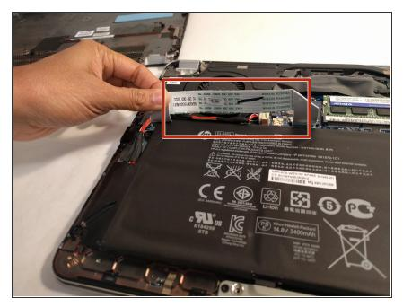
Once the device is open, move the ribbon cable to the side.
