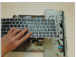
Separate the metal case from the keyboard by peeling off the tape that connects them.
