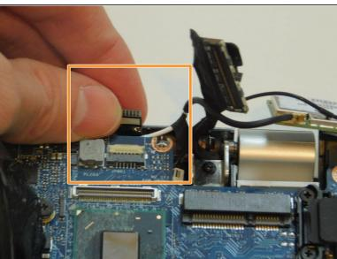
• Using the plastic spudger, remove the power button cable. This is the small, purple ribbon cable at the back of the motherboard.
