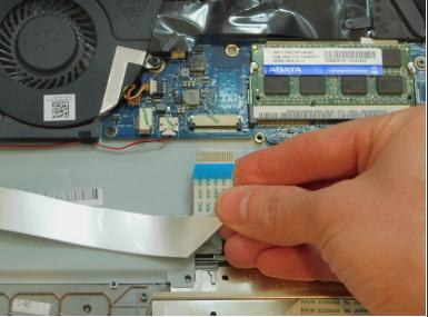
Disconnect the ribbon cable running to the ports on the right-hand side of the laptop.
