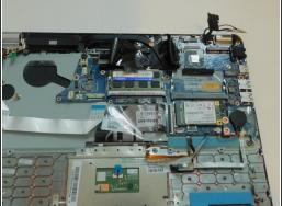
Using a Phillips #0 screwdriver, remove any remaining screws attaching the motherboard to the rest of the laptop.
