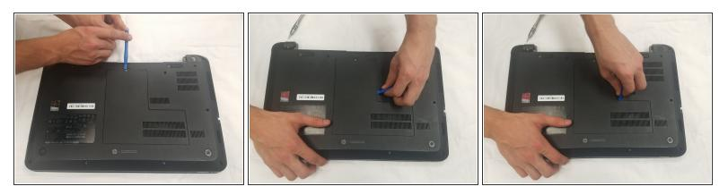
• Using a plastic opening tool, pry the back panel from the computer, going all the way around it.
