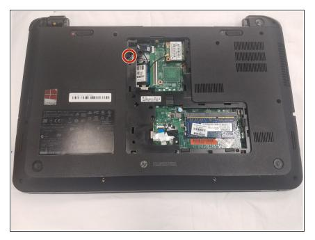
Once you have removed the panel there is one screw (2.5x6mm) that will need to be unscrewed.
