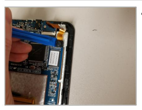
The rear-facing camera module of the tablet is secured to the device with a strong adhesive. Insert your plastic opening tool underneath the rear-facing camera module and gently pry it up until it is released from the glue. You may now remove the entire camera assembly.
