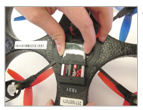
Pull the battery away from the slot to remove it.
