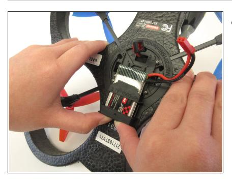
Push the battery upward with your thumbs to loosen it from the tight slot until your thumbs can not reach the bottom of the battery anymore.
