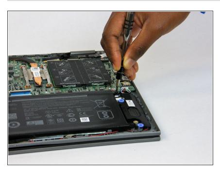
Remove the four 3mm Phillips #0 screws at the corners of the battery that secure it to the laptop.
