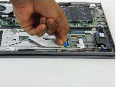
• Undo the clasps that hold the ribbon cables in place. Then, remove the ribbon cables.
