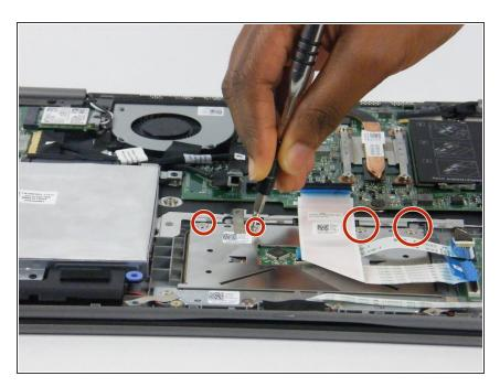
Remove the 1.5mm Phillips #0 screws that hold the touchpad to the laptop case.
