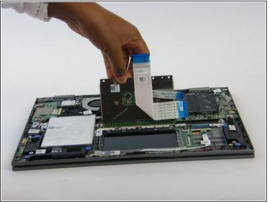
Push up on the touchpad to release it from the housing. Then you can remove the touchpad.
