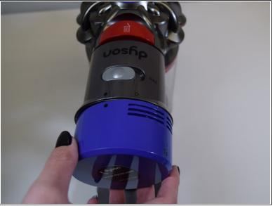
• Twist the HEPA filter to the left, matching up two black dots on the device and pulling away.
