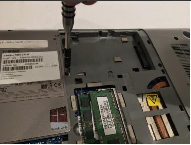
Using a Philips #0 screwdriver, unscrew the 1.5mm screw located near the left edge of the opening near the mother board.
