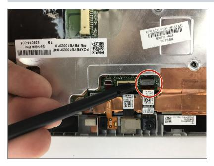
Begin by removing the ribbon that connects the front facing webcam to the motherboard. You can use a black nylon spudger as pictured to do this.
