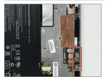
The HP Spectre X2 Has three Cameras: A front facing webcam( blue arrow), a rear Facing webcam (orange arrow), and a 3d camera (red box). The 3d camera is covered by tape that connects to the heat sink.
