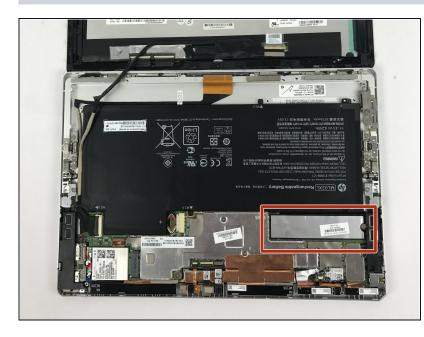
• Once you have successfully removed the screen, locate the solid state drive (SSD).
