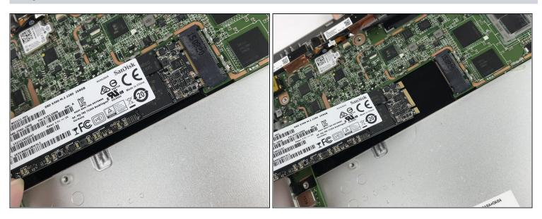
• Carefully, pull the SSD out of the slot at an angle.
