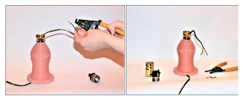
• Strip off 1/2" of the insulation with the wire stripper and twist the wire strands together by hand.
