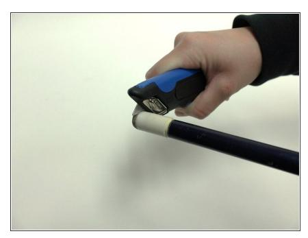
Remove the old, worn tip using a box cutter. Make sure that the old tip is completely removed.
