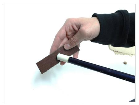
Sand down the end of the pool stick using the sand paper until the surface is flat and smooth.
