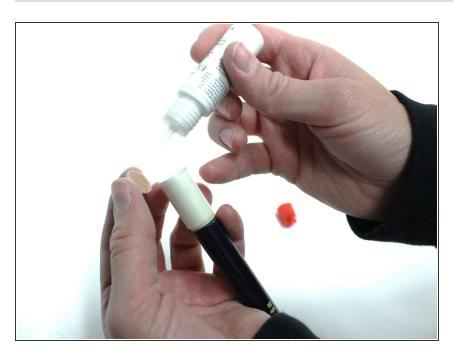
Glue the sanded side of the new side of the new tip to the end of the pool tip.
