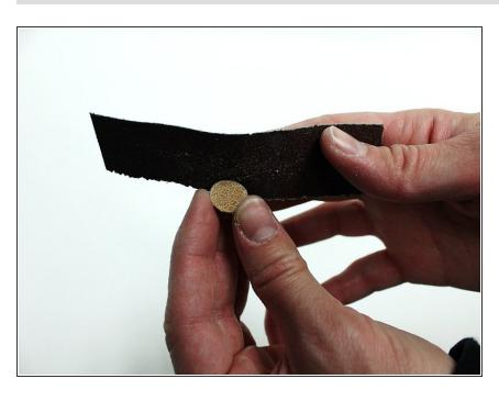
Use the sandpaper to file the edges and backside of the new tip.
