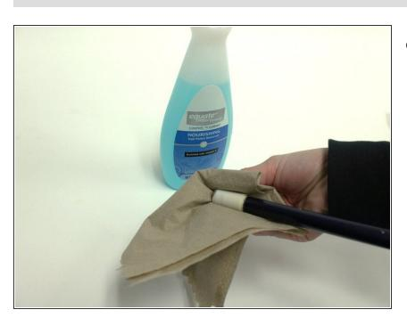
Remove any old glue or gunk using a napkin soaked with nail polish remover.
