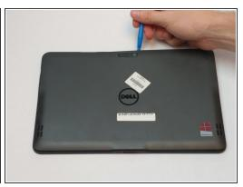
Using the blue opening tool, separate the back plastic cover from the device. Start in a corner, and work your way around the tablet.
