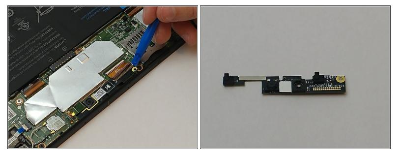
Gently lift up the camera using the plastic opening tool and remove it from the tablet.
