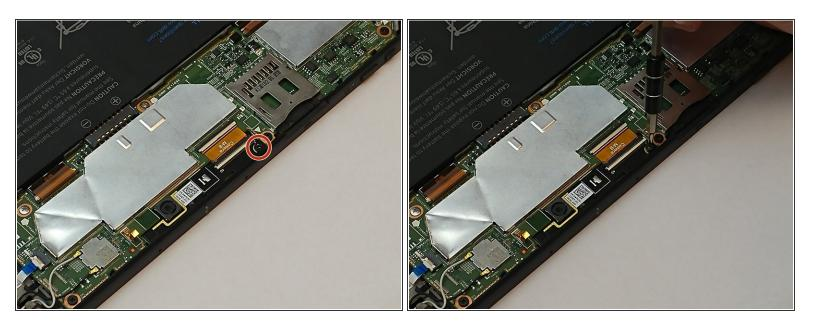
Using a JIS #00 screwdriver, remove the one 4.0mm screw securing the camera to the motherboard.
