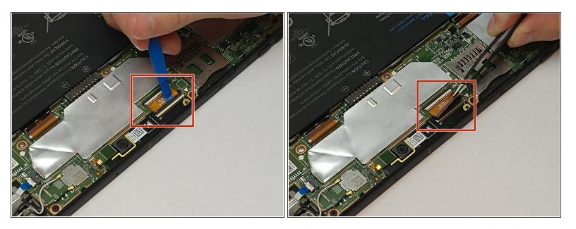
• Use an opening tool to release the black clamp. With the tweezers gently lift and disconnect the motherboad from the camera.
