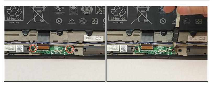
• Using a JIS #00 screwdriver, remove the two 4.0mm screws securing it to the motherboard.
