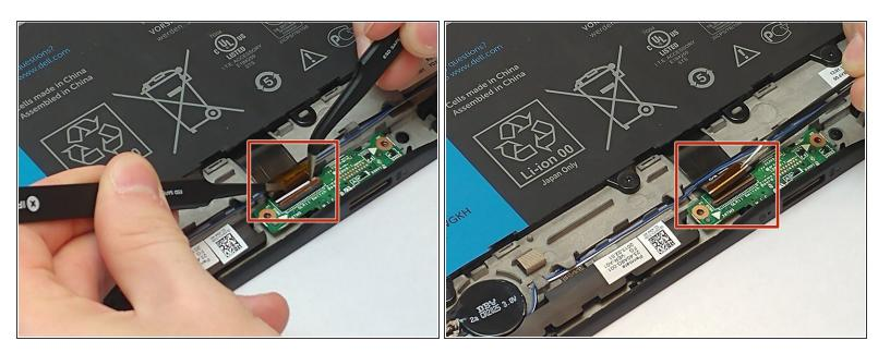
Lift up the orange clamp connecting the black DOC B/D cable to the charging board.
