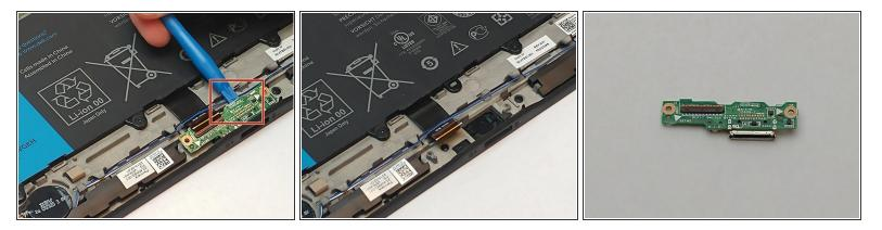
Place the opening tool underneath the charging board, lift up, and slide it out the charging port, along with its board.
