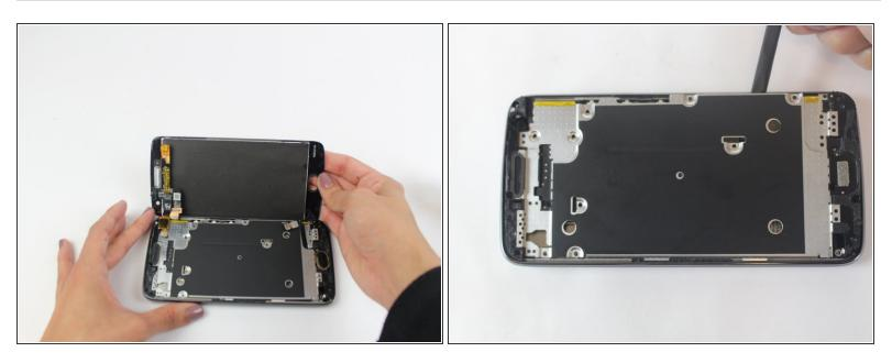
• Remove the interior metal covering using the plastic opening tool.
