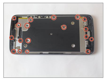
Using a size 000 Philips head screwdriver, unscrew the nineteen 4 mm screws. Yellow tinted kapton tape will need to be removed to get to some of the screws.
