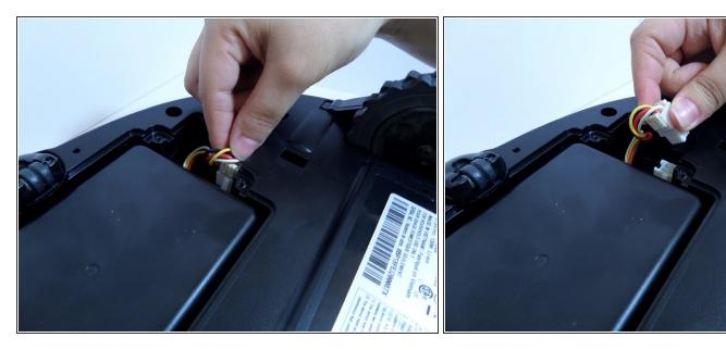
Using one hand, pinch the white plastic connector where the battery's wiring connects the POWERbot. Pull up to disconnect.
