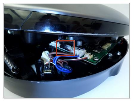
Pinching the top and bottom of the black wired connector, pull outward, fully detaching the top from the bottom of the device.
