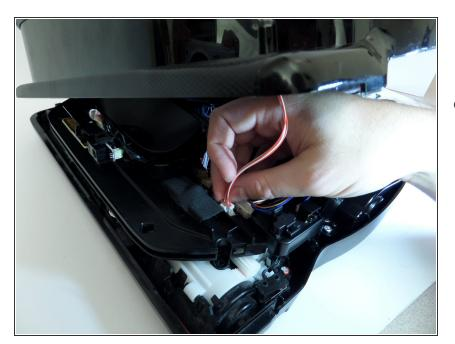
Disconnect the white and red wired connector attached to the top half of the base of the vacuum by squeezing the connector and pulling up.
