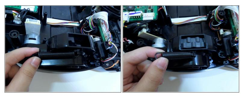
• With the spring fully retracted, unhook the spring from the wheel casing.
