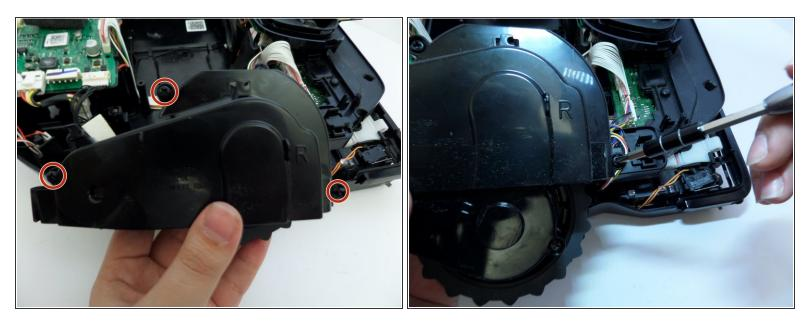
• Remove the three screws fastening the two halves of the wheel casing together.
