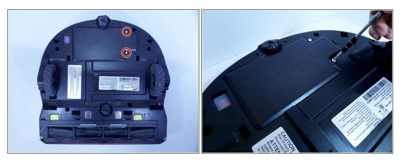
• Remove the two exposed screws on the top right of the device.
