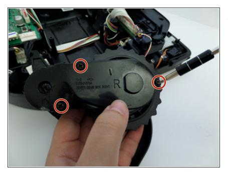
Remove the three screws on the remaining half of the wheel casing.
