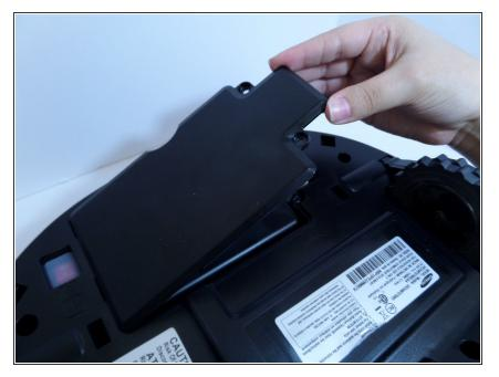
• Lift the cover plate to expose the battery.
