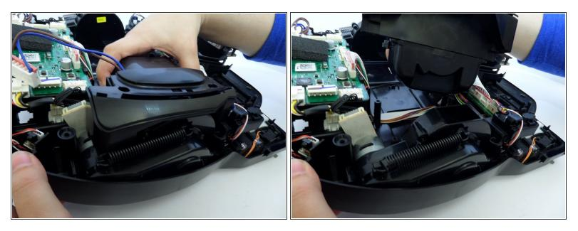
• Lift the motor by grabbing the body of the motor, lifting upward.
