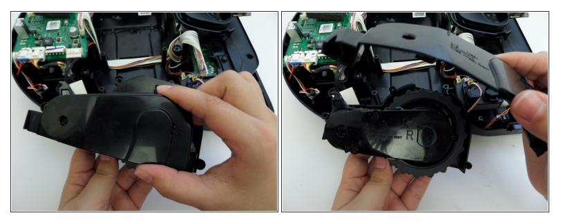
• Separate the unsecured half of the wheel casing, exposing the wheel.
