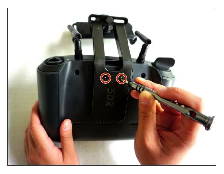
Using the PH0 Phillips head screwdriver, unscrew the two screws located above the 3DR logo.
