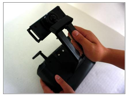
Hold the controller with one hand, and the phone holder with the other hand. Pull the phone holder upward, away from the controller.
