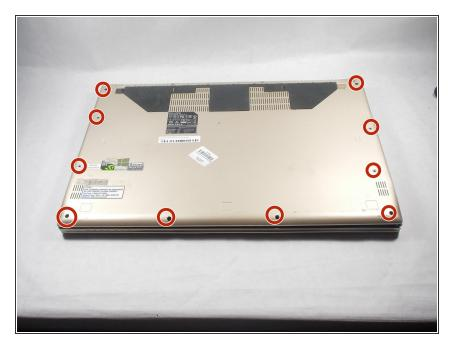
Using the screwdriver, unscrew the highlighted 1.2mm Phillips head #0 screws which secure the back panel into place.
