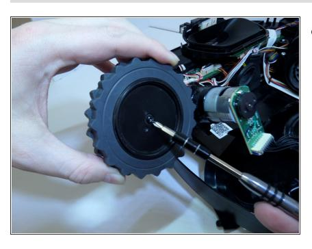
Unscrew the black 1 cm screw securing the center of the wheel to the remaining half of the wheel casing.
