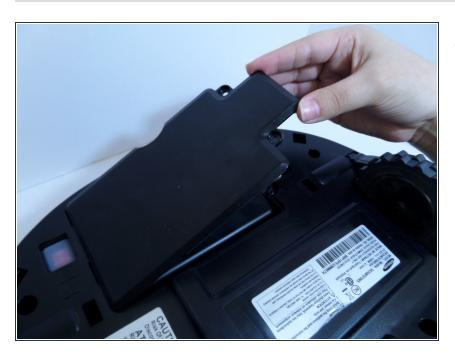
Lift the cover plate to expose the battery.
