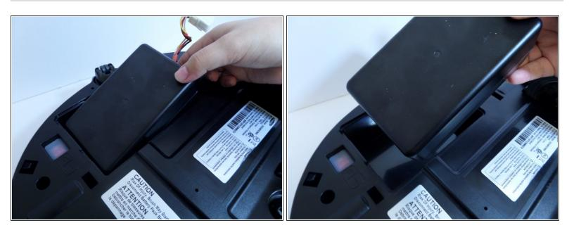
Lift the battery from the right side, up and out of its compartment.
