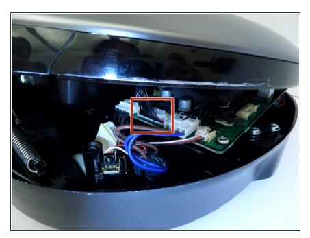
Pinching the top and bottom of the black wired connector, pull outward, fully detaching the top from the bottom of the device.
