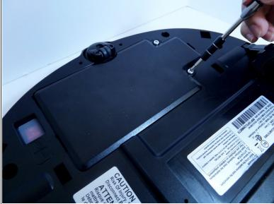
Remove the two exposed screws on the top right of the device.
