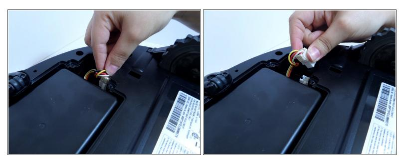
Using one hand, pinch the white plastic connector where the battery's wiring connects the POWERbot. Pull up to disconnect.
