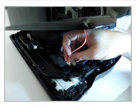
Disconnect the white and red wired connector attached to the top half of the base of the vacuum by squeezing the connector and pulling up.
