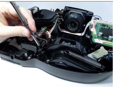
Unscrew the two screws securing the left and right ends of the wheel casing to the base of the vacuum.
