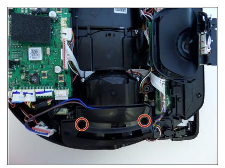
Remove the two 1.5 cm screws on the motor chamber.
