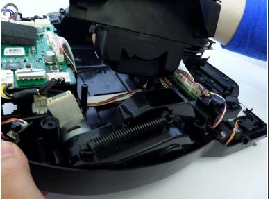
• Lift the motor by grabbing the body of the motor, lifting upward.
