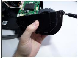
Remove the screws that are fastening the two halves of the wheel casing together.
