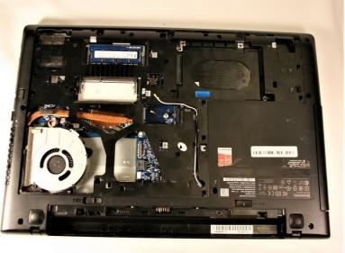
Slide the cover away from the hinges and lift the panel off.
