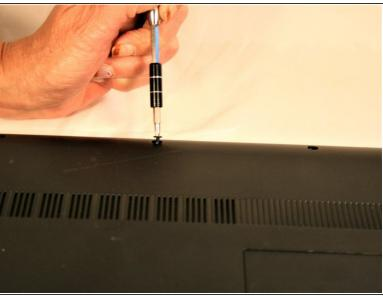
Remove the three screws securing the outer cover of the laptop using a Phillips #0 screwdriver.
